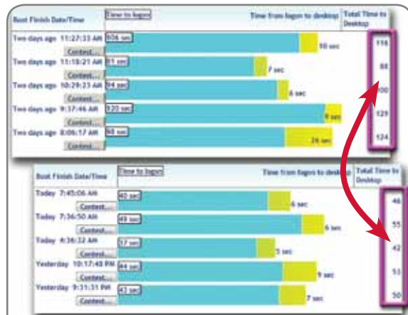
Using BootRacer utility for Windows, we timed a series of boot-up tests of our workstation with and without the HyperBoot facility in Diskeeper 12 Professional enabled. Using HyperBoot, the average time needed to boot our workstation to the Windows desktop dropped by 56%.
